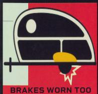
THIN MAY CAUSE METAL TO METAL **CONTACT WHICH CAN** CAUSE A SPARK.
